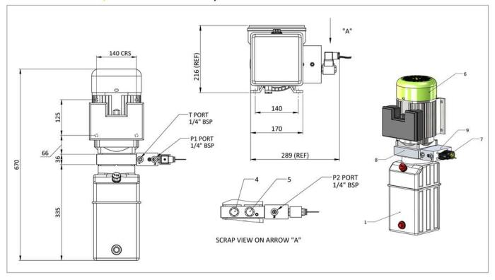
Electric Motor: 1Ph 1.5Kw 1450rpm
