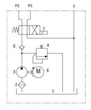
The tower lift pack is designed to control power to two independent hydraulic circuits preventing any possibility of operator error. The stabilizer rams are deployed via a lever valve and only at this point can the tower be raised as the change over is interlocked. Again the stabiliser rams cannot be adjusted until the tower is lowered.
